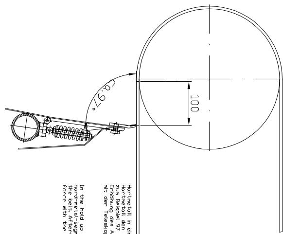
In the hold up position you must mount the hard metal segments with angle of 90° to the belt. Afterwards you can change the force with the telescope.
