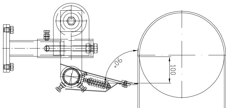
During using the hard-metal-segments shall move to 90° angle to the belt.
