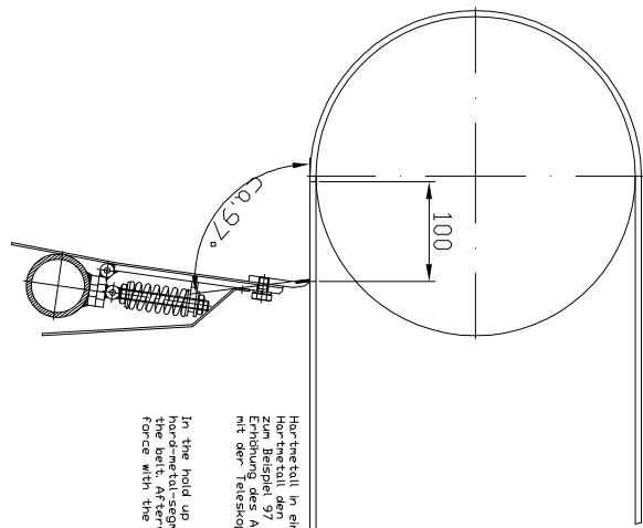
In the hold up position you must mount the Hartmetall so that it is at 90° to the belt. Afterwards you can change the force with the telescope.
